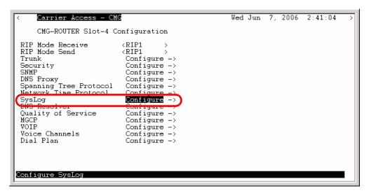
2. To enable **SysLog** (System Log Message Service), scroll **<Disabled>** to **<Enable>**, with the **[SPACEBAR]**, select **[ENTER]**.
